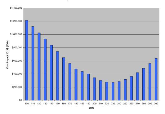
It is noted by reviewing the chart that the optimum level, based solely on quantitative analysis, is approximately 230 MW. The proposed total level of 185MW (with 80 MW coming from AMPGS), while not optimal, is more economical than lower alternatives, based upon the increased cost of market purchases.
