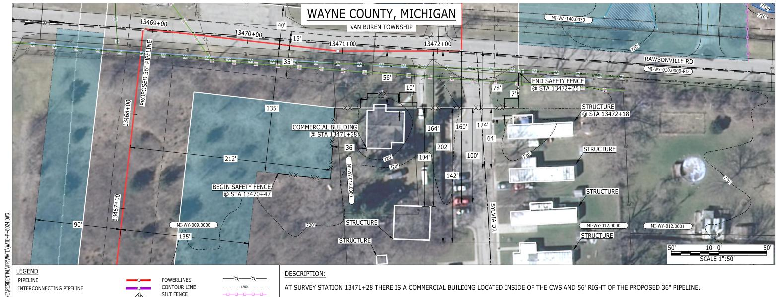
AT SURVEY STATION 13472+18 THERE IS A STRUCTURE LOCATED 7' TO THE RIGHT OF THE CWS AND 78' RIGHT OF THE PROPOSED 36" PIPELINE.
